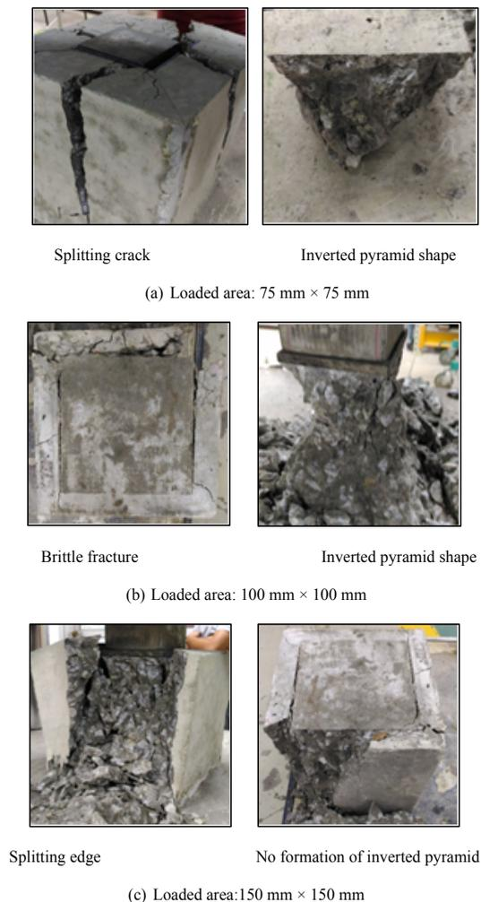
Figure 5. Modes of failure for different steel plate dimensions
