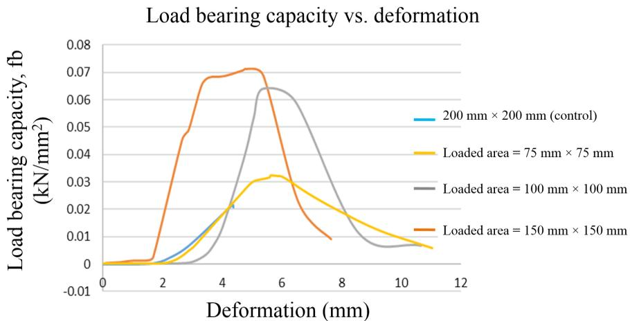
Figure 3. Graph of load bearing capacity (kN/mm<sup>2</sup>) versus deformation (mm)
